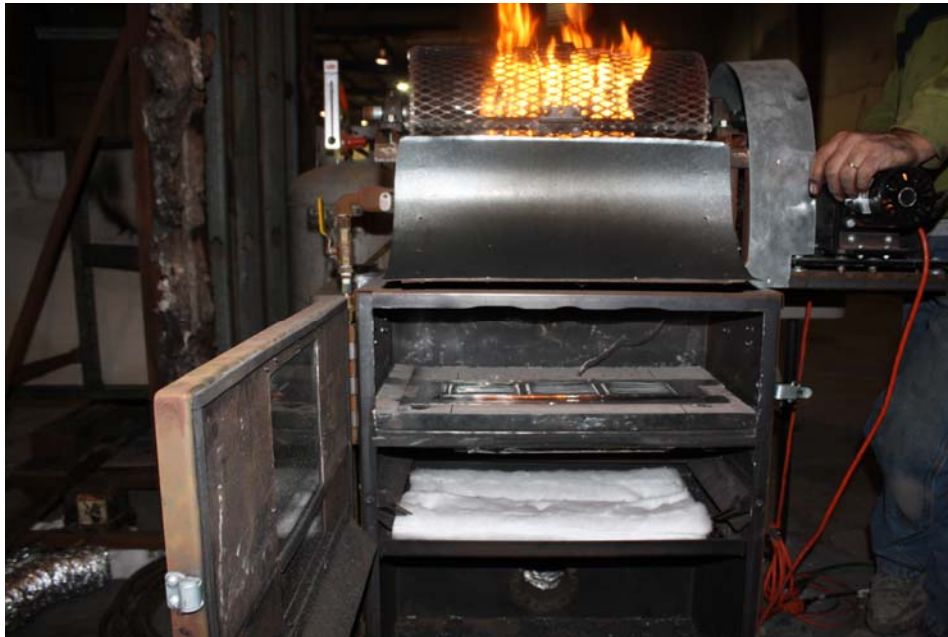
Immediately prior to ember exposure: Brands exposed to igniter for 3 minutes
